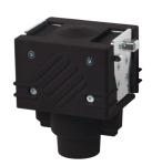
The MagnetGripper can be used to grip ferromagnetic parts. The maximum weight of a flat component that can be gripped with the MagnetGripper is 300 g. It is recommended to test the intended handling of the component several times, as the alloy, surface finish and shape of the component determine the maximum weight. It is also recommended to grip the component at or above the component's center of gravity, if possible, in order to avoid center-of-gravity-dependent torques.
